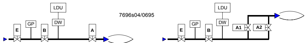
Plants without vent pipe to atmosphere
